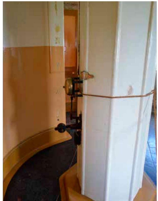
LEFT TOP: The clockwork mechanism that rotated the optic in the lantern of the South Foreland High Light. Like all mechanical clocks, it needed the keepers to wind it, in this case, 100 turns of the winding handle to keep the rotation going for about 2\frac{1}{2} hours. LEFT BOTTOM: The winding of the clock raised a weight suspended on a wire on the inside of a tube at the centre of the lighthouse. As the clock ran down, the weight fell to the bottom whereupon it was time to wind it back up to the top. RIGHT TOP: The octagonal tube containing the clock weight occupies the centre of the tower and predominates in the lower room of the lighthouse. RIGHT BOTTOM: The tube is also present in the service room (below the lantern room), of course, where a bell is mounted so as to give warning to the keepers when the clock needs to be rewound.
